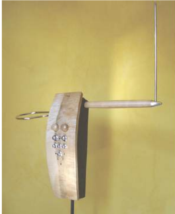
Theremin seen from the perspective of the performer.
