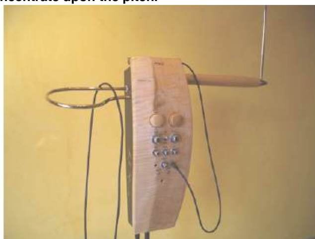
The cable upon the horizontal antenna stops the sounding of the theremin.
