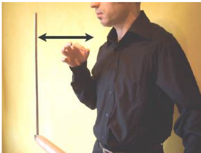
We use the vertical antenna on our right to produce different pitches, according to how near or far from it our right hand and arm are.
