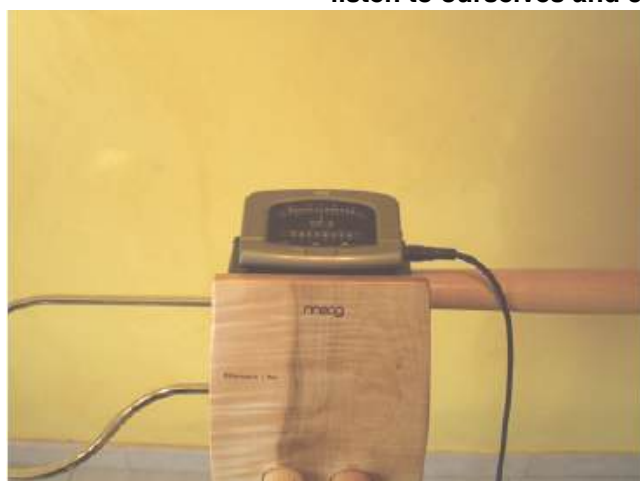
Tuning indicator [chromatic tuner] connected to the theremin to visualize the notes, even when the instrument does not sound through the speaker.
